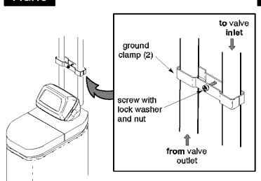
FIG.17 WATER METER JUMPER WIRE
